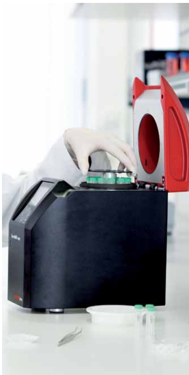
Guaranteed safety during homogenizing due to bayonet catch.
