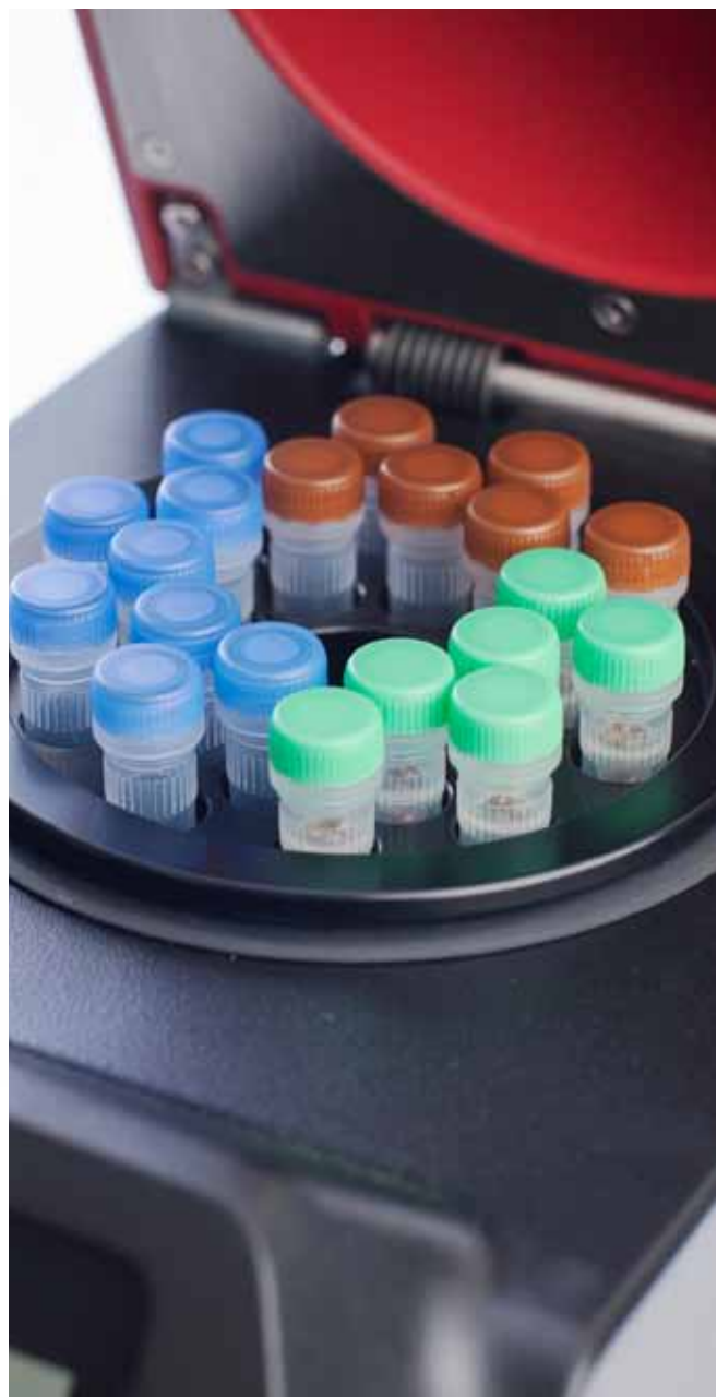
Exchangeable sample adapters enable an easy sample handling.
